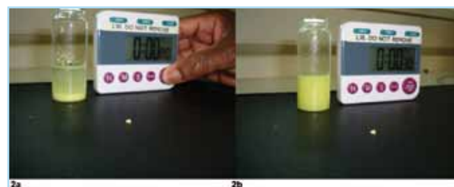
Figure 2. Photographs showing granule dispersibility in 10 ml of water (a) undispersed and (b) dispersed after 30 seconds.
